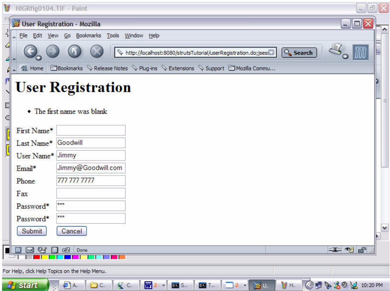
Figure 1.5 User Registration JSP with validation errors
